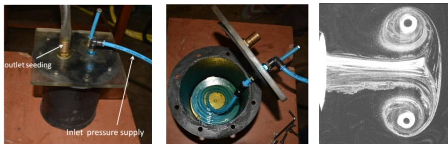
Figure 2: Inexpensive seed generator for PIV developed with C. L. Dora, K. K. Bharadwaj (Ph D Students), Particle image of a vortex ring obtained using inexpensive seed generator
