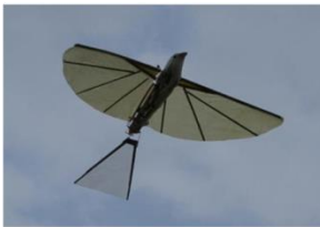
Weight : 30 g Span of each wing =25cm Endurance: 10-12 mins Design Cruise speed : 6 m/s
