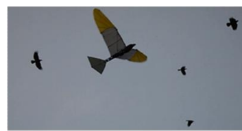
• wingspan 1.6m • Dry Weight :400 grams • Endurance : more than 1 hour with 2 batteries( 1000mAh each 3cell) • Cruise speed: 6 to 8 m/s
