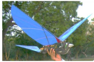
Weight : 260 g Span of each wing =50cm Endurance: 30-35 mins Design Cruise speed : 6 m/s
